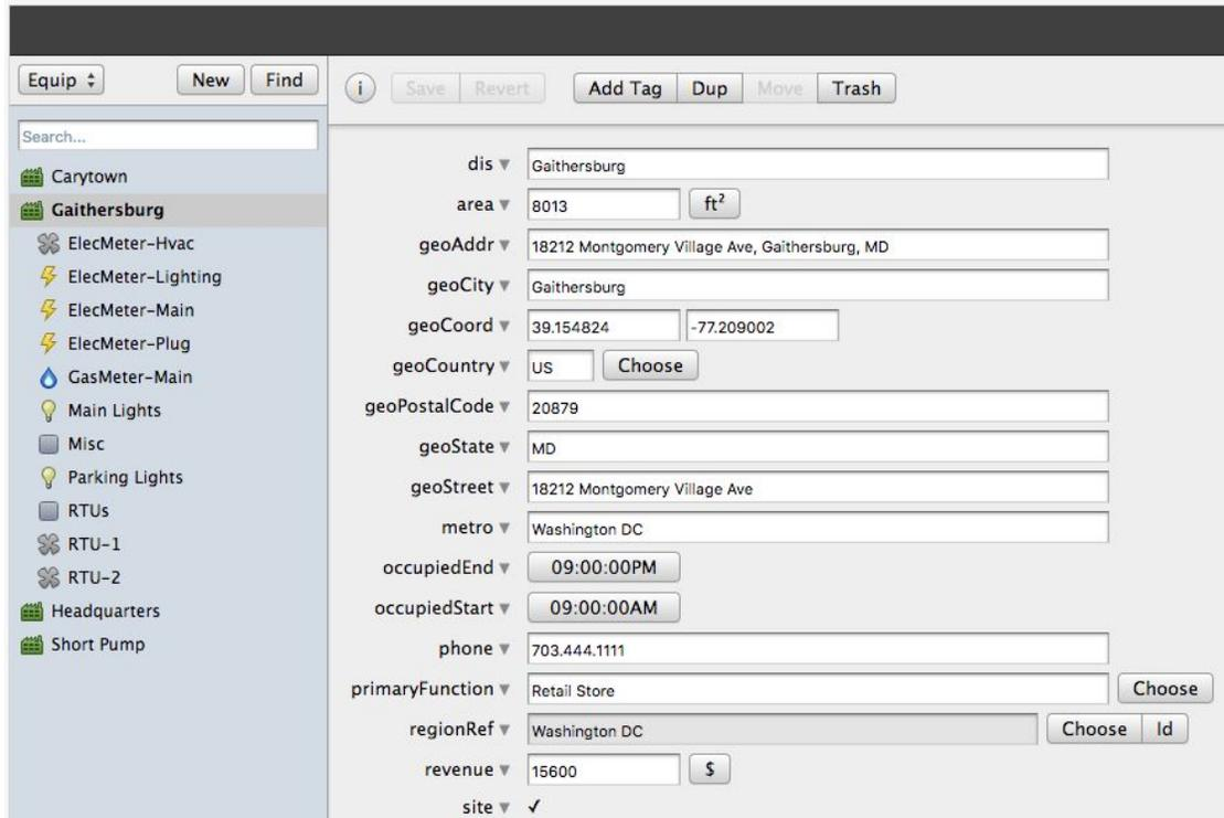
The screenshot shows the Project Haystack interface. On the left is a sidebar with a search bar and a tree view of locations. The 'Gaithersburg' location is selected, showing a list of equipment types like 'ElecMeter-Hvac', 'ElecMeter-Lighting', etc. The main area is a form for editing an entity. The form has a toolbar with buttons for 'New', 'Find', 'Save', 'Revert', 'Add Tag', 'Dup', 'Move', and 'Trash'. The form fields include:
